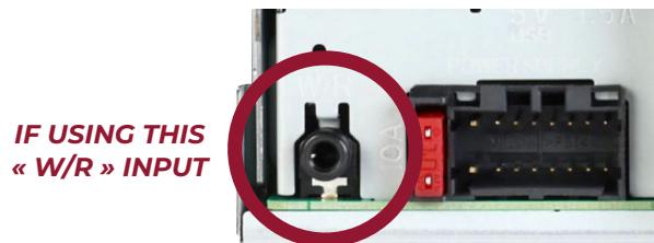
When using a stand-alone steering wheel interface connected to our **DMH-WT6000NEX** via the « **W/R INPUT** » jack (Wired Remote Input), **you must now enable the communication** which is by default set to «OFF».
